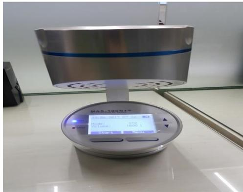
Gambar 3.11 Microbial Air Sampler (MAS)
